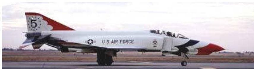
The F-4's conversion was the most extensive in the team's history. Among other modifications, paints that had worked on the F-100 made the F-4 look patchy because of multicolored alloys used in the F-4 to resist heat and friction at Mach II speeds. As a result, a polyurethane paint base was developed and used to cover the problem. The white paint base remains a part of today's Thunderbird aircraft.
